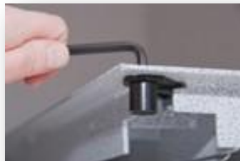
Use Allen key to adjust leveling screws
